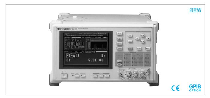
The MP1552A is a portable analyzer designed specifically for troubleshooting SDH, PDH, and ATM network construction and maintenance as well as for evaluating equipment for these networks. Various systems can be configured according to the application using plug-in units.
